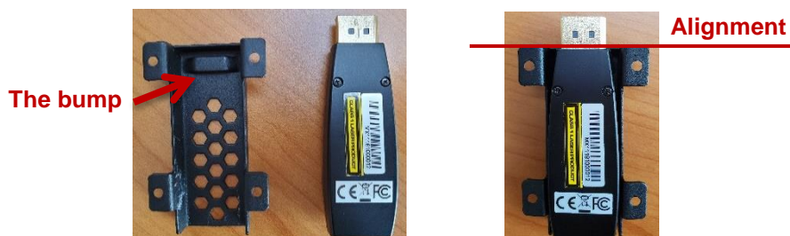
Fig. 2: Insert the push button into the bracket
