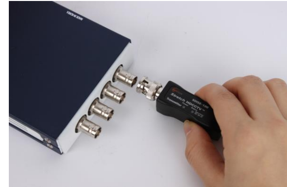
Figure 2 – TX module of SDISE-100
