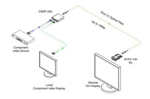
Figure 1 – Connection Diagram of CNDF-200
