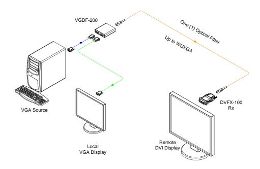
Figure 1 - Connection Diagram of VGDF-200
