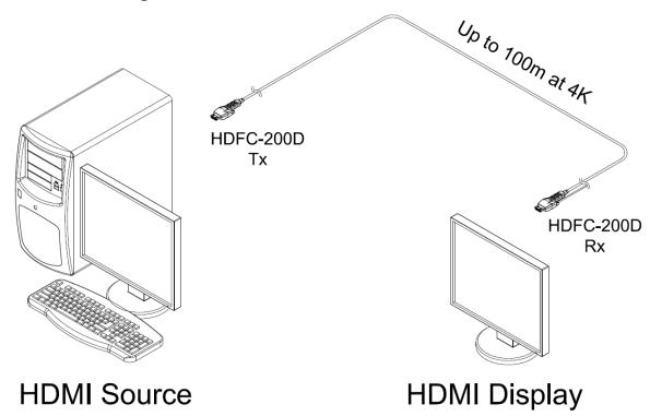
Example : PC to HDMI Monitor Set-up
