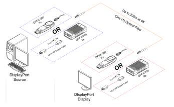
Figure 1 – Overall Connection of DPFX-700-TR
