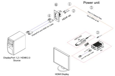
① Connect Power cables into 3-pin power connector of HDHF-4K.
